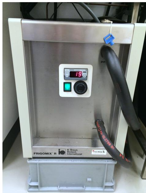
The peltier controller is the device shown above. There is no need to change settings directly on this device, all of the settings are controlled via the software. The red light on the front panel will flash when the peltier is active (i.e. it has been instructed to control the temperature by the software).
