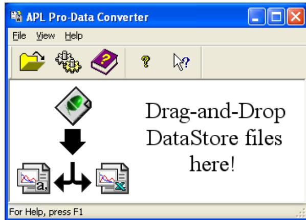
To convert files to .csv for use in other graphing software, open the APL Pro-Data Converter application. Drag and drop files from the Windows Explorer (file manager) onto the window shown and a converted file will appear in the same directory as the original file.
