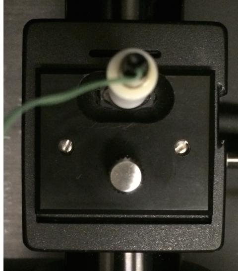
Place the cell holder, cell and probe into the hole in the Peltier jacket (f) in the sample compartment.
