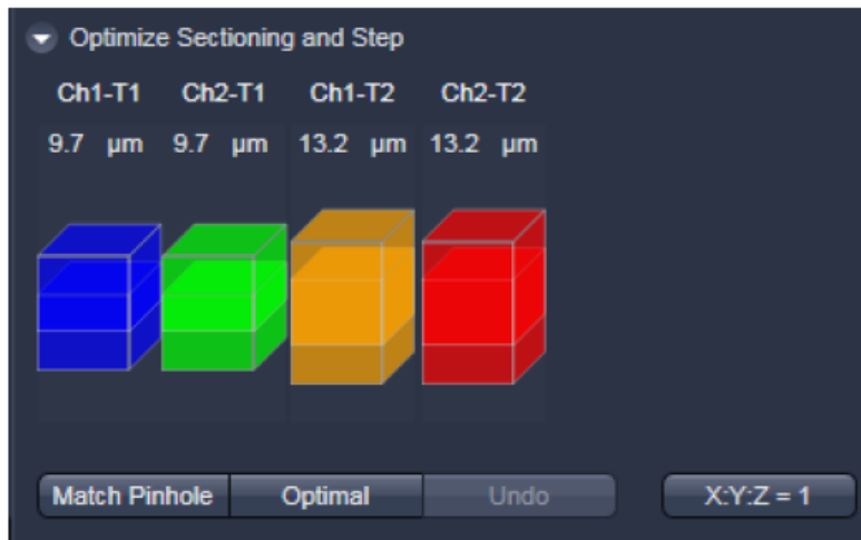
Fig. 77 Optimize Sectioning and Step: Optimal Interval is set starting with one Airy unit for all channels
