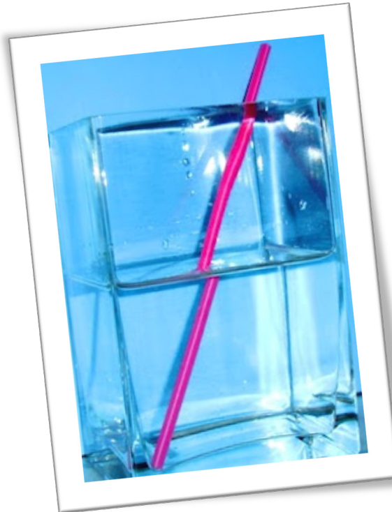
A refractive index mismatch gives rise to geometrical aberrations.
