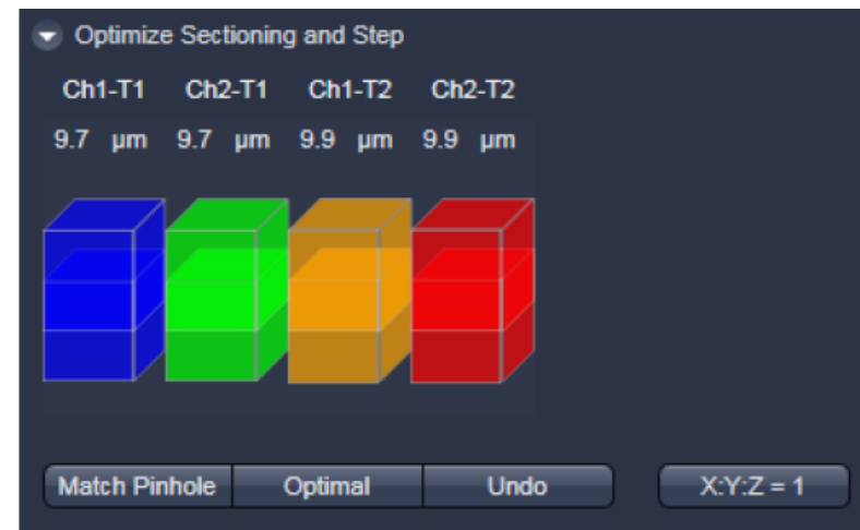
Fig. 78 Optimize Sectioning and Step: Match Pinhole to Step resulting in equal optical sections for all channels
